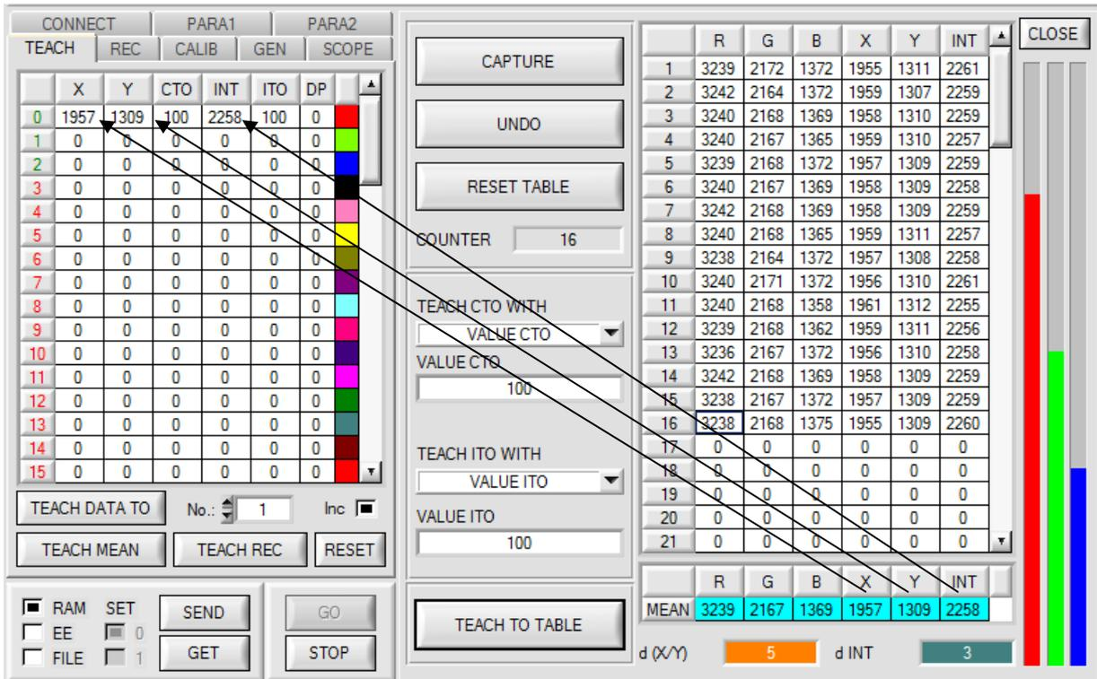
The screenshot shows the 'TEACH MEAN VAL' panel. It features a main data table with columns X, Y, CTO, INT, ITO, and DP. A 'COUNTER' is set to 16. Below the main table are controls for 'TEACH CTO WITH' and 'TEACH ITO WITH', both set to 'VALUE CTO' and 'VALUE ITO' respectively, with a value of 100. A 'TEACH TO TABLE' button is at the bottom. To the right, a 'MEAN' table shows the calculated mean values for each parameter. A vertical bar on the right indicates color and intensity deviations.
